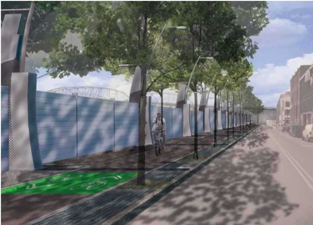
Figure 23: Streetlight bases at the edge of a park form supports into which removable flood barriers slot in.
